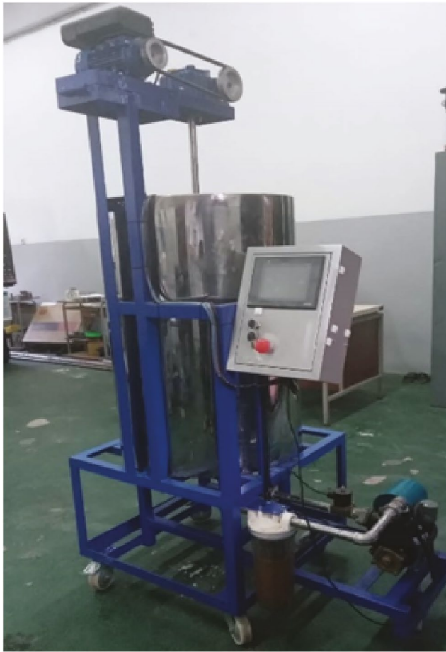
Figure 3: Coffee cherry grading machine semi-wash and full-wash method.
