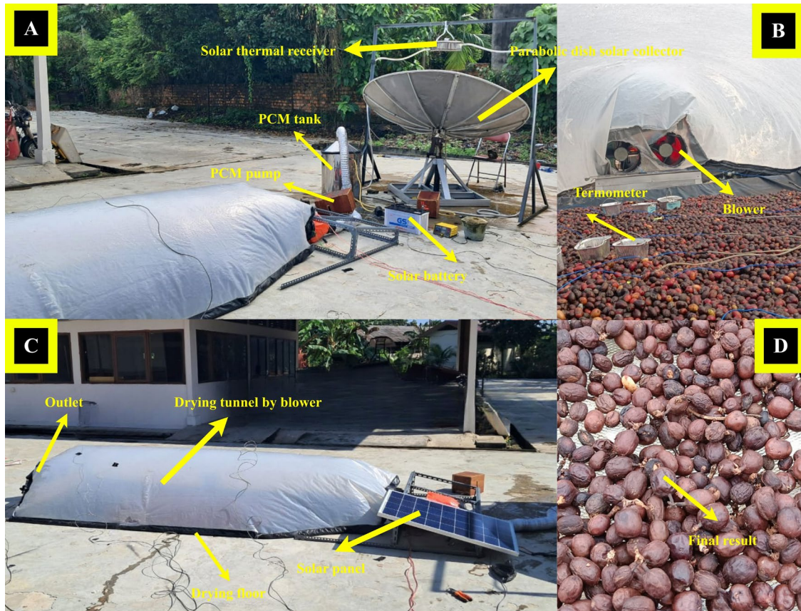
Figure 1: Photographs of the experimental parabolic solar dryer facility showing (a) the back view, (b) the interior, (c) the right-side view, and (d) the dried coffee cherries.
