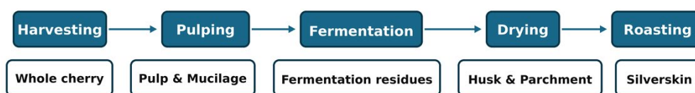
Figure 2: Coffee processing chain and generation of major by-products.
